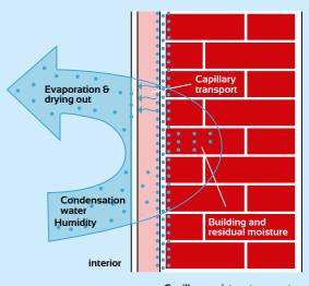
Capillary moisture transport to the inner surface, drying out is possible!
